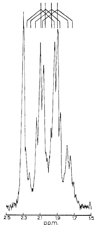
Figure 2.—Phosphine methyl resonances of trans - [\text{Pt}(\text{CNC}_2\text{H}_5)_2\{\text{P}(\text{CH}_3)_2(\text{C}_6\text{H}_5)\}_2\{\text{C}(\text{NHC}_2\text{H}_5)\text{CH}_3(\text{NHC}_2\text{H}_5)\}](\text{PF}_6)_2 recorded on a \text{CH}_2\text{Cl}_2 solution at 31^\circ with an HA100 spectrometer using a sweep width of 500 Hz, showing four nonequivalent phosphine methyls and the anilino methyl at \delta 2.31. The scheme indicates platinum coupling to the phosphine methyls and phosphorus coupling is omitted for clarity.
